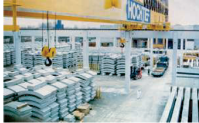
Fig. 8.60. The 64 ton crane of Hochtief Corp. uses fuzzy PLC based antisway positioning control (Video)
